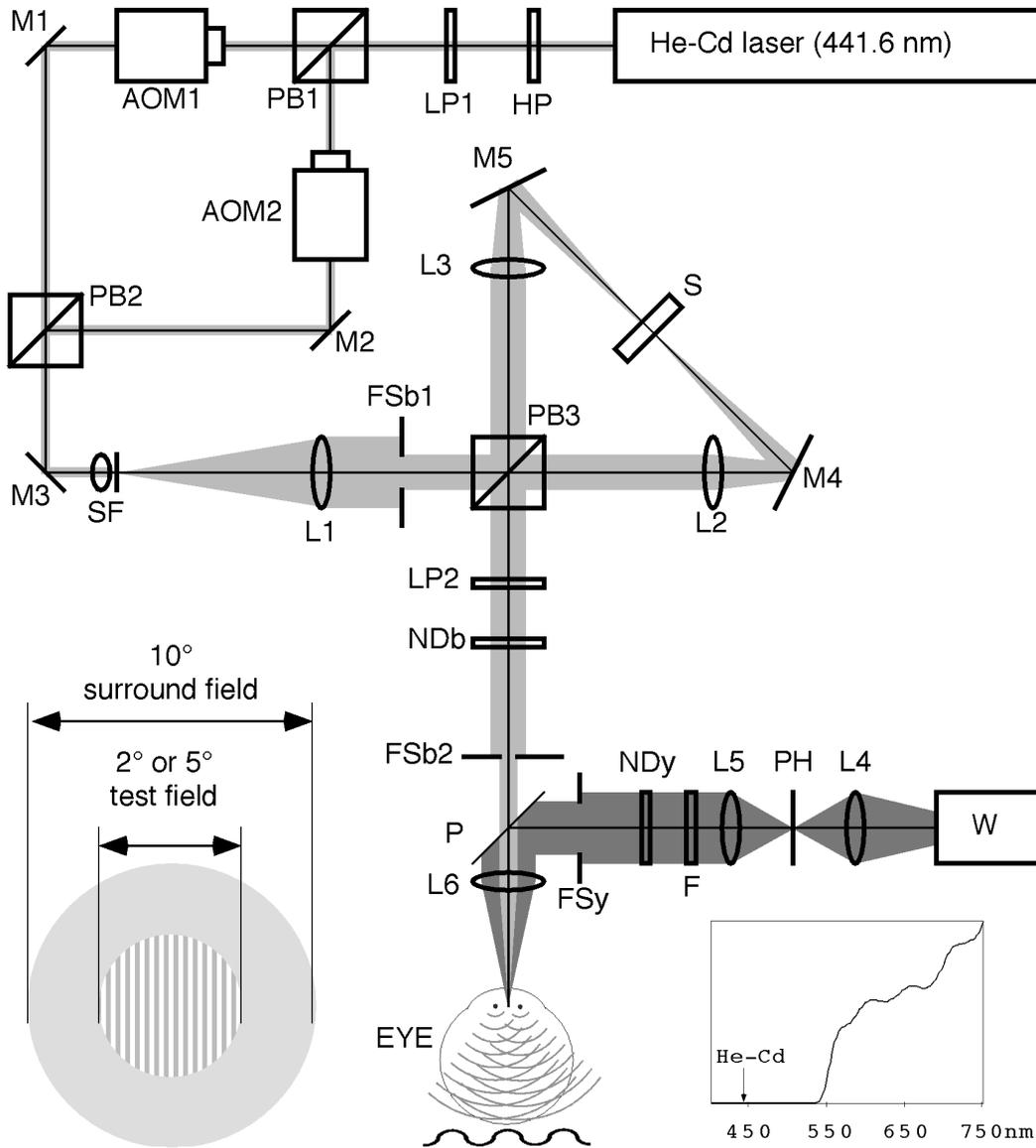
**Fig. 1.** Two-channel Maxwellian view apparatus used to deliver high contrast S-cone isolating gratings. One path incorporates a 441.6-nm helium–cadmium laser interferometer to generate gratings, and a second path introduces a bright yellow adapting light to selectively reduce responses from L- and M-cones. See text for details.
