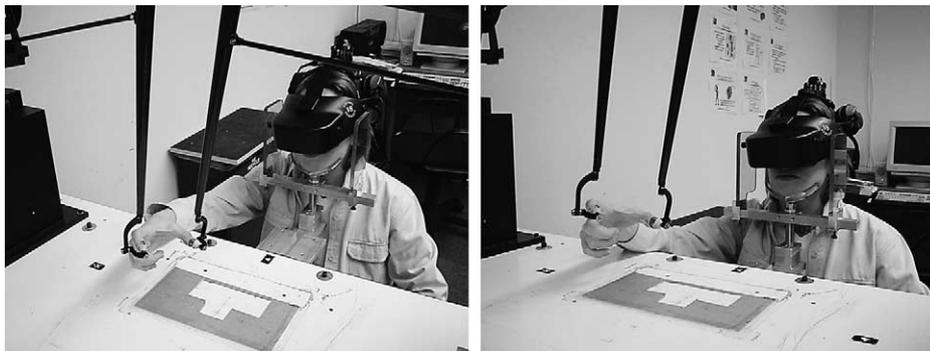
Fig. 1. A subject is shown in the experimental apparatus. Visual stimuli were delivered via a head-mounted display, and haptic stimuli were delivered via the force feedback devices attached to the subject's thumb and index fingers. The subject is grasping two (virtual) fronto-parallel surfaces, with her thumb against the front surface and her index finger wrapped around behind the back surface.
