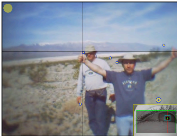
Figure 5. Moving target method of five-point calibration. Observers who were tracked outdoors followed a partner's moving thumb, which paused at positions that create a five-point calibration (indicated by overlaid circles).
